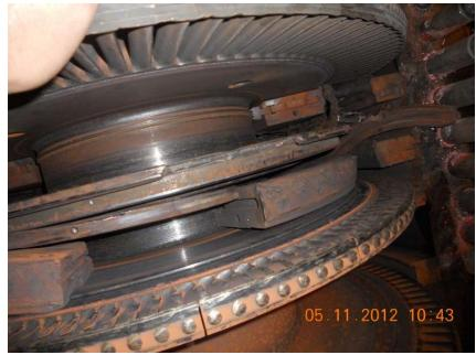
Corrosion deposits on steam turbine rotor
