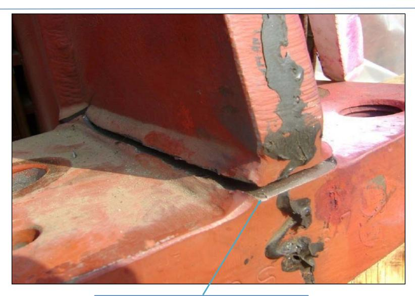
Crack developed in welding of stator foot
