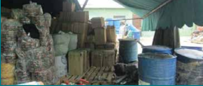
Poor Risk Segregation between flammable chemicals and dispatch stocks
