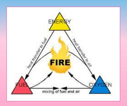
Energy (heat) causes vaporization of fuel in and results in thermal decomposition in presence of Oxygen (Chemical Reaction)
