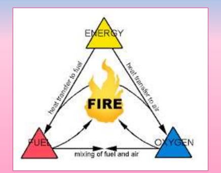
*Energy (heat) causes vaporization of fuel in and results in thermal decomposition in presence of Oxygen (Chemical Reaction)*
